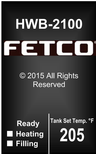
First Screen: Unit started: And is Filling and Heating
